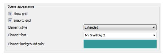
The Show grid, Snap to grid, Element style and Element font parameters affect the view of a workflow:
