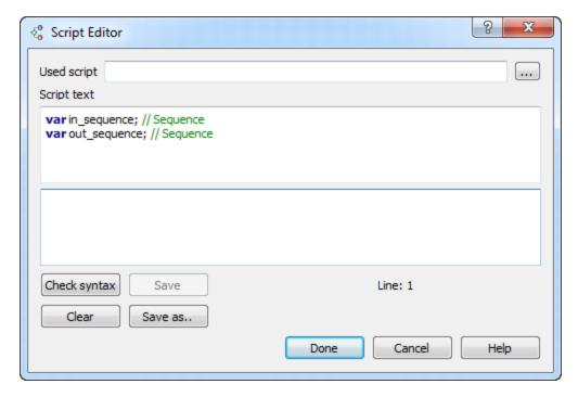
As you can see there are predefined variables for the ports and the attributes in the script. The variables for the input slots begin with the "in\_" prefix, variables for the output slots begin with the "out\_" prefix. It is possible to load a script from a file (use the *Used script* field to do it).
