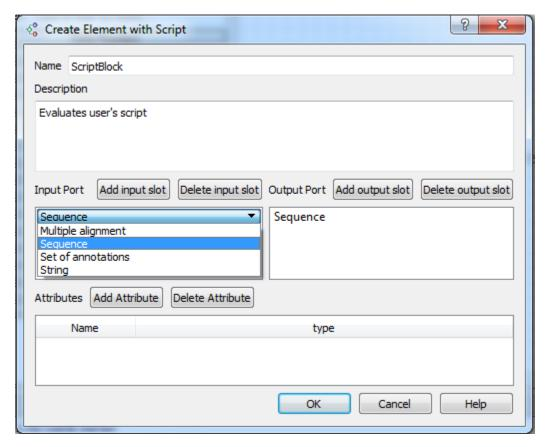
Here you should set the name of the element, its description and input / output ports of the element. It is possible to create a port with several input / output slots
