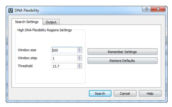
The calculation is made for overlapping windows along a given sequence. If there are two or more consecutive windows with an average flexibility threshold (in each window) greater than the specified *Threshold* parameter, such area is marked by an *annotation*.
